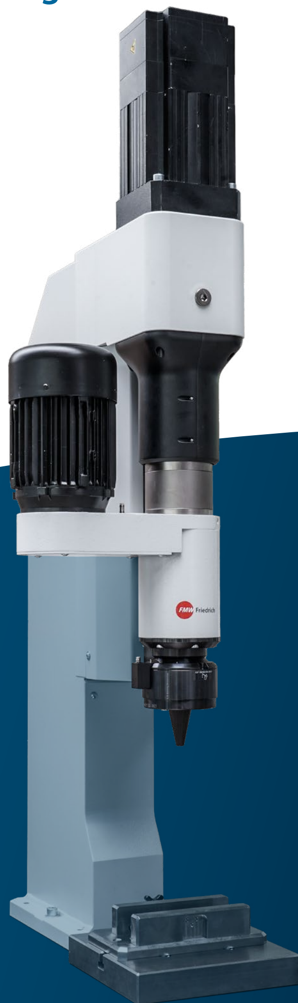
Servo-NE with projection and length measurement
