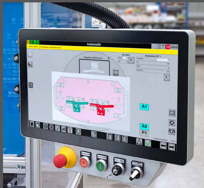
Example (see photo): A base size error of a component to be riveted is shown in red.
